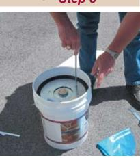
To remove the follow plate from an empty or partially full container, insert the handle rod into the open nut on the surface of the plate and pull it out.
