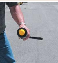
Attach the end cap and cone tip to the end of the barrel. Make sure the tip of the cone is cut to the diameter of the bead you want to apply.
