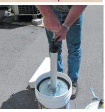
Depress the rod release lever and draw back the rod with a smooth, even pull. Make sure the barrel stays flush with the plate and don't tilt the gun as you pull the rod back.
