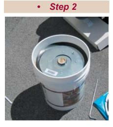
Place the follow plate on top of the chinking in the pail making sure that there is a good seal between the wall of the pail and the flexible edges of the follow plate.
