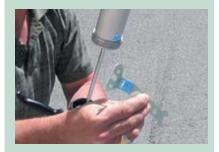
If the gun begins to suck air, tighten the blue base with the wrench that comes with the gun.
