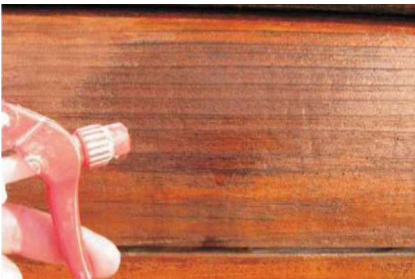
Water absorbing into a wood through a finish that is no longer water repellent
